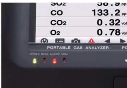
Unit status is clearly displayed on the LEDs on the front of the unit.
